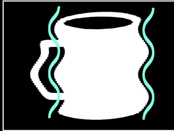
Image read from rolling shutter sensor
