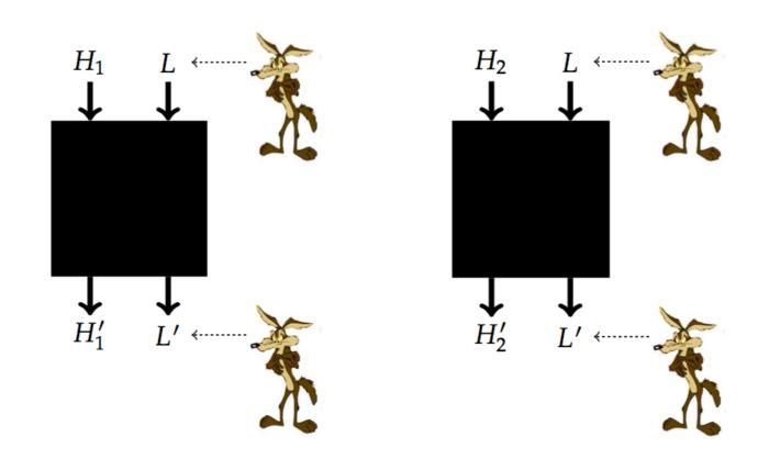
$\forall s_1, s_2, s_1', s_2', \quad s_1 \sim s_2 \land (P, s_1) \Downarrow s_1' \land (P, s_2) \Downarrow s_2' \implies s_1' \sim s_2'$
